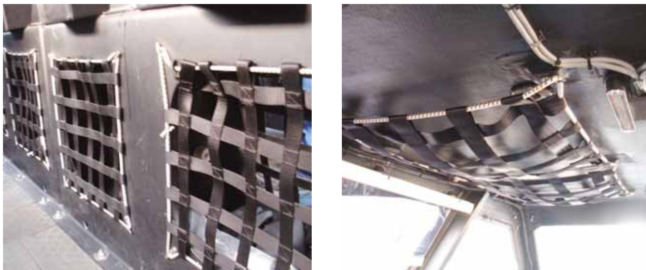
Figure G-3 Examples of under-seat and roof storage utilised on a HSC.
