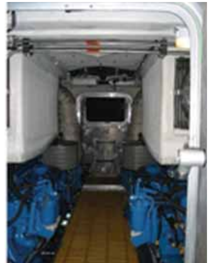
Figure H-2 Examples of good access around engines – RNLI Tamar Class Lifeboat (left) and USN SEALION-I Technical Demonstrator (right).
