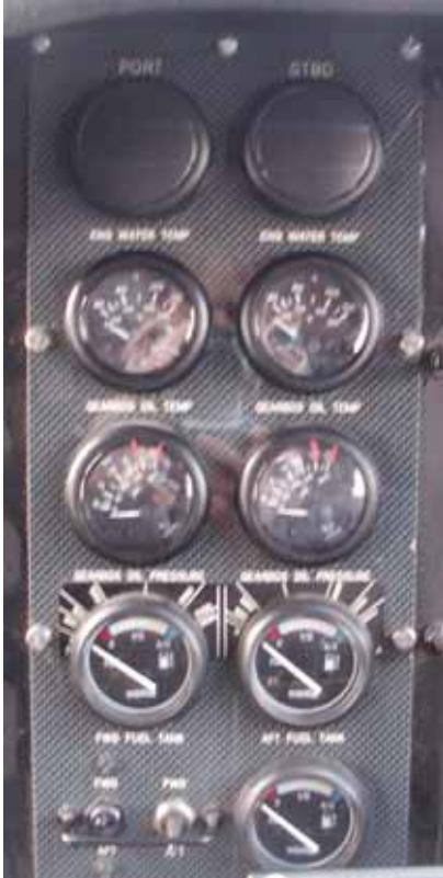
Figure F-8 An example of multiple engine instruments (twin engine) arranged in columns for easy comparison.
