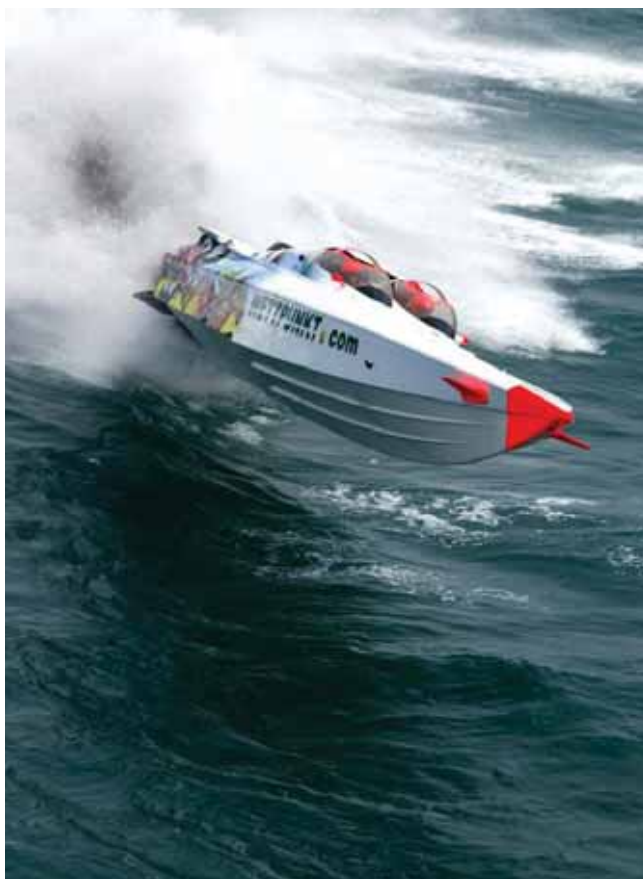
Figure A-4 An example of how a HSC often lands on its side thus resulting in an impact with a considerable lateral component ( g_X ) in addition to a vertical component ( g_Z ), where g_Z equates to the axis perpendicular to the HSC deck.
