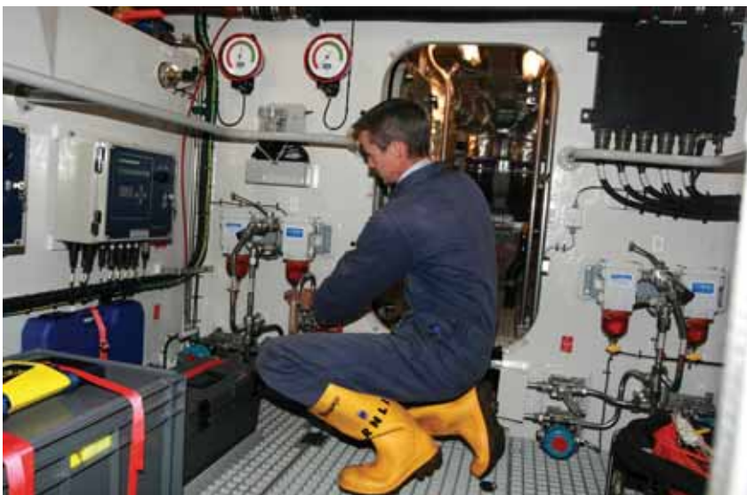
Figure H-1 Example of good access to service components, e.g. fuel filters Image copyright: RNLI
