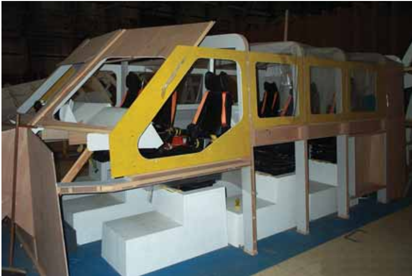
Figure I-5 Example of RNLI Mock-Up used during the design review process.
