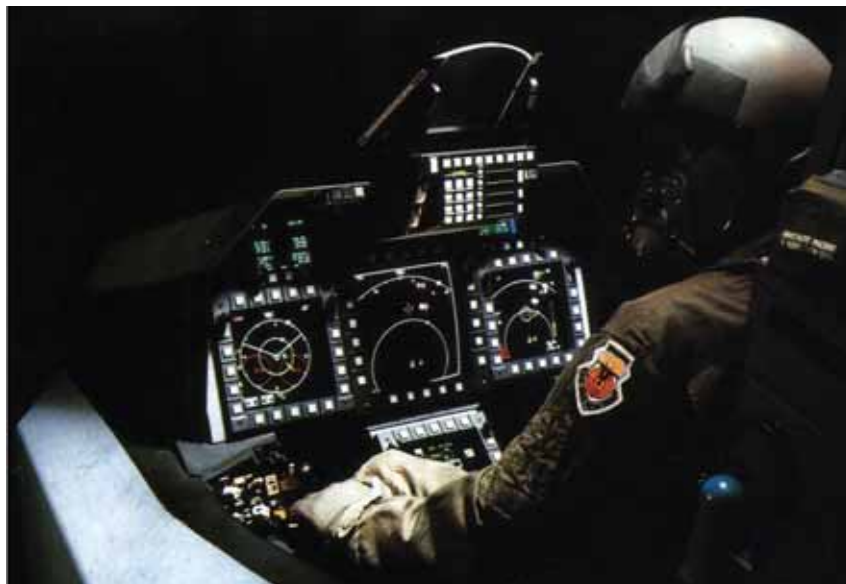
Figure 4-2 F22 mock-up being used to assess cockpit ergonomics Source: www.simpits.org
