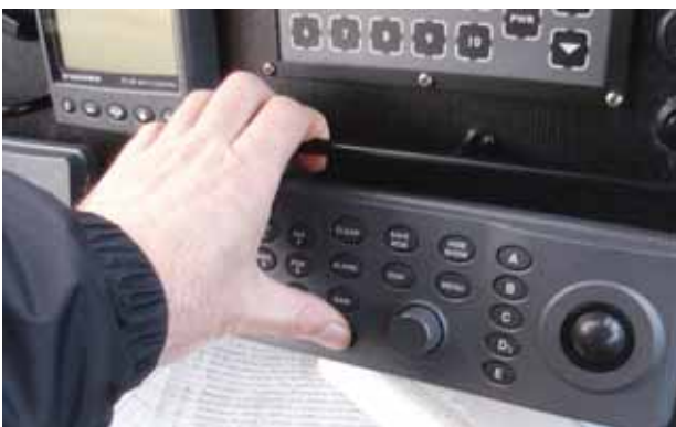
Figure F-13 An example of the use of a 'rail' to steady the operators hand when using equipment/switches/trackball in a harsh motion environment.
