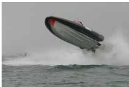
Figure A-5 An extreme example of a HSC rolling whilst operating in choppy sea conditions
