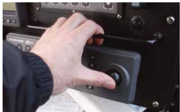
Figure F-13 An example of the use of a 'rail' to steady the operators hand when using equipment/switches/trackball in a harsh motion environment.
