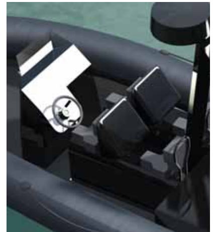
Figure I-2 (Below) Example of a 3D CAD image of a HSC crew workstation demonstrating how the overall cockpit concept may work.
