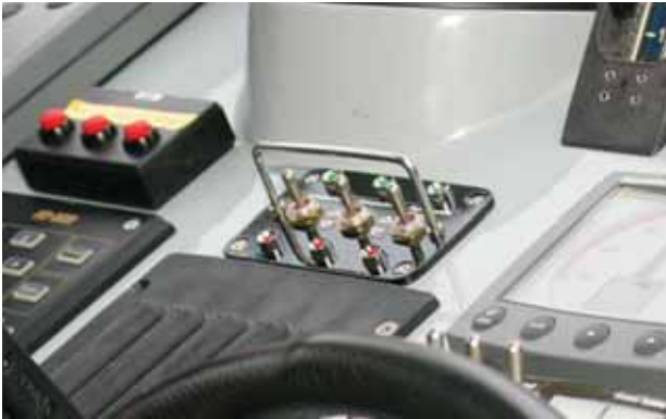
Figure F-12 An example of a guard over switches to stop accidental operation when operating HSC in a harsh motion environment.
