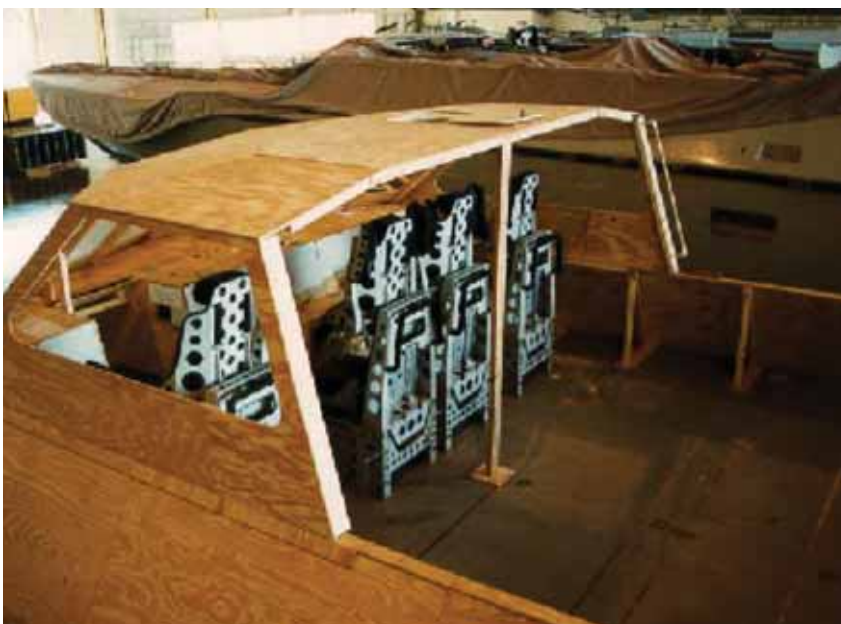
Figure I-7a Mock-up of USN MkV SOC being used to establish locations and spacing of crew seats, external view, etc.
