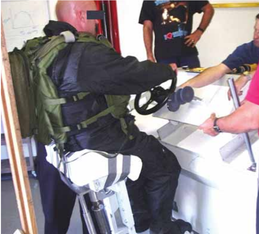
Figure I-6a Example of Helm console mock-Up being used to develop the MMI to work with a prototype suspension seat.
