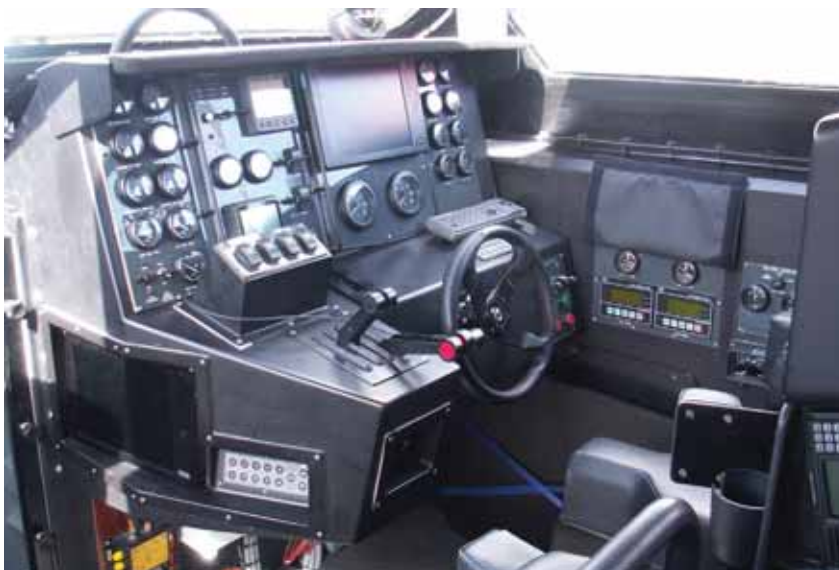
Figure I-8b A view of the resultant layout of the UK Fast transit Craft Helm position
