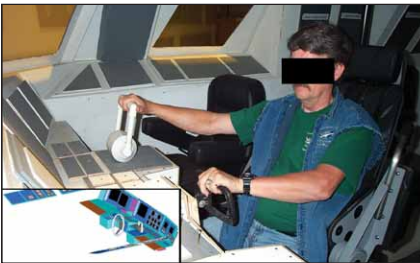
Figure K-4 Images of the SEALION-I Coxswain's CAD Console, mock-up and actual cockpit
