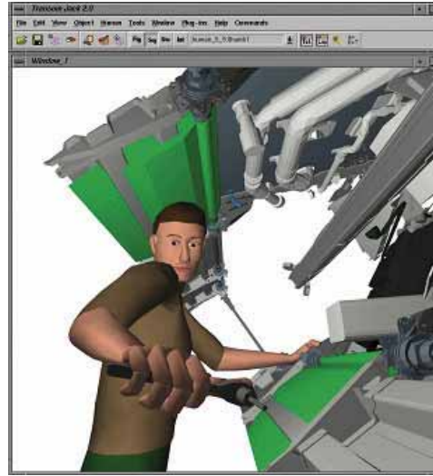
Figure I-4 An example of how CAD modelling can be used to assess the interaction between the HSC systems and the operator/maintainer.
