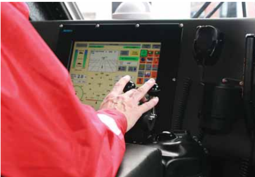
Figure F-1 An example of HSC Man-Machine Interface design solutions. The RNLI Tamar Class Lifeboat engine throttles are operated via finger-tip control; also visible are the trackball and its control buttons to the right of the throttle controls, SIMS display screen, radio microphone and cup-holder.
