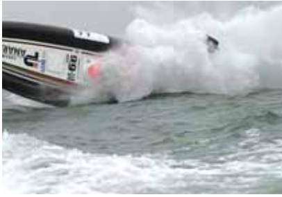
Figure E-1 RIBs, which are inherently more stable than other high-speed monohulls are still at risk of capsizing in certain conditions.
