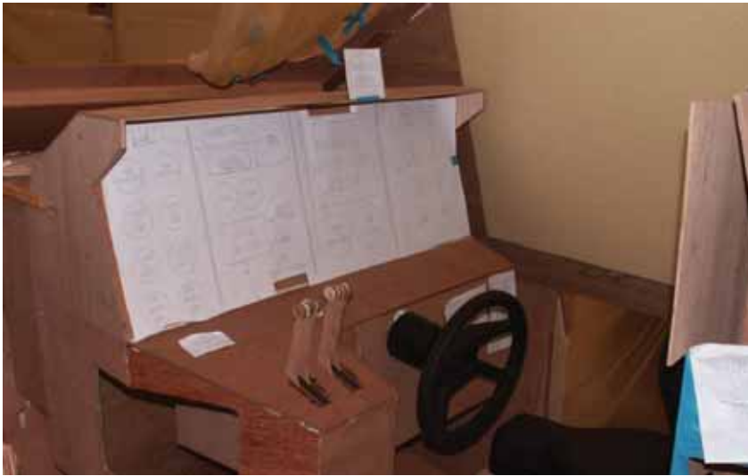
Figure I-8a mock-up of a UK Fast Transit craft helm position being used to establish locations and spacing of crew seats, external view, control locations and instrumentation layout etc.
