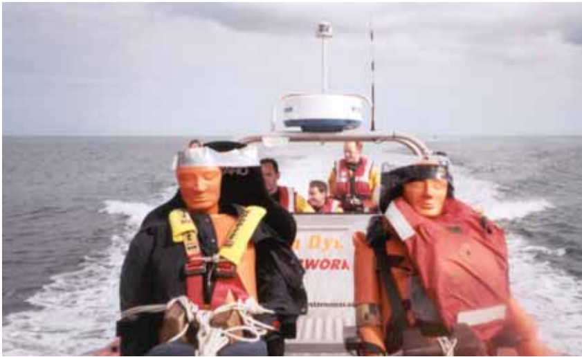
Figure J-7 Example of anthropometric dummies being used for the testing of the RNLI/Fraser-Nash suspension seats and the subsequent assessment by RNLI personnel.
