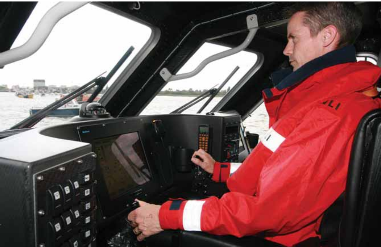
Figure F-17 Example of coxswain using arm-rest mounted throttle (right hand) and tiller (left hand) controls on the RNLI Tamar Class Lifeboat.
