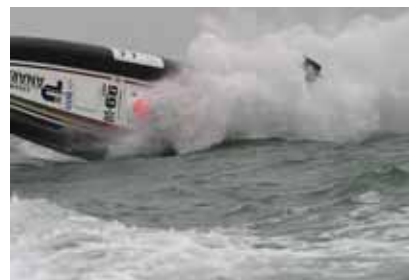
Figure A-5 An extreme example of a HSC rolling whilst operating in choppy sea conditions
