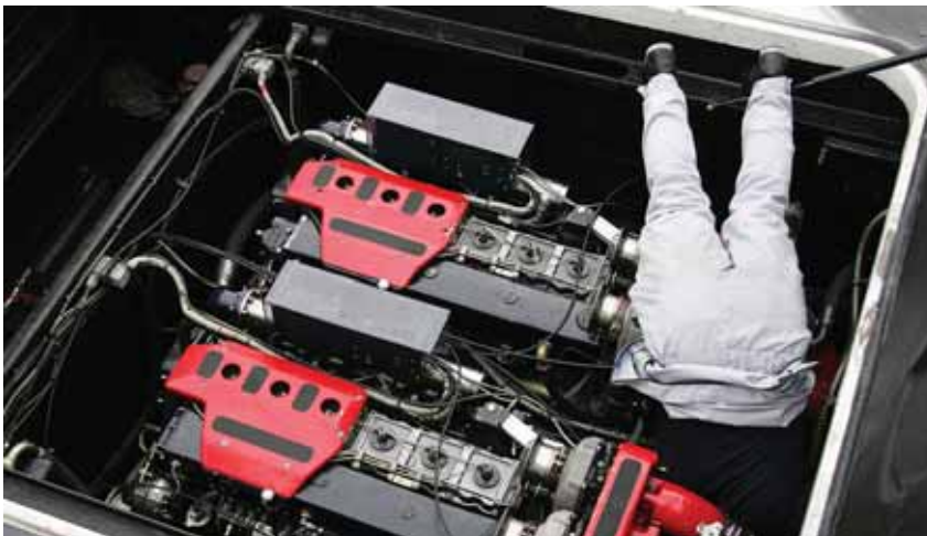
Figure H-3 Example of poor access to engine components
