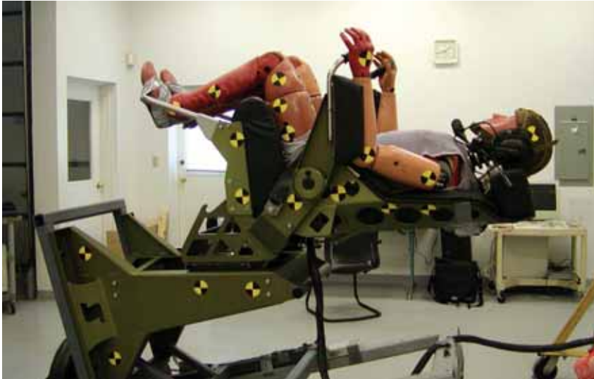
Figure J-5 Example of an anthropometric test dummy being using for the testing of the Stidd/Taylor V5 suspension seats on a deceleration (crash) track. Image copyright: University of Virginia
