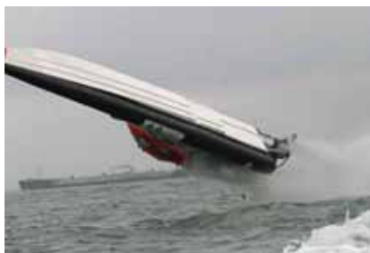
Figure A-5 An extreme example of a HSC rolling whilst operating in choppy sea conditions
