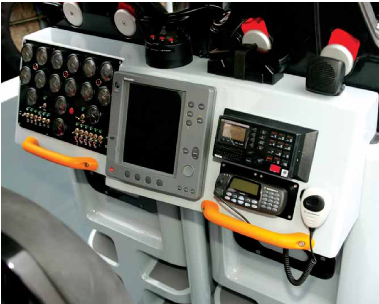
Figure E-3 Example of hand holds (shown in yellow) used to help HSC occupants to maintain their postural stability
