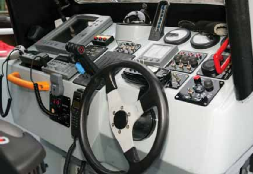
Figure F-2a An example of a coxswain and navigator workstation showing console/instrument layout. Image copyright: FB Design
