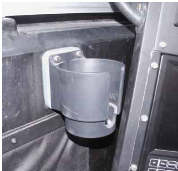
Figure G-2 Example of a cup holder, and its secondary use for general storage (e.g. communications headset, hand-held VHF radio, etc.).
