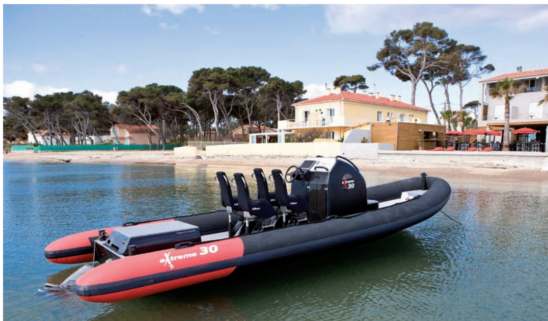
The hull has a relatively shallow deadrise for this size of RIB and at first glance the shape does not appear technically advanced
