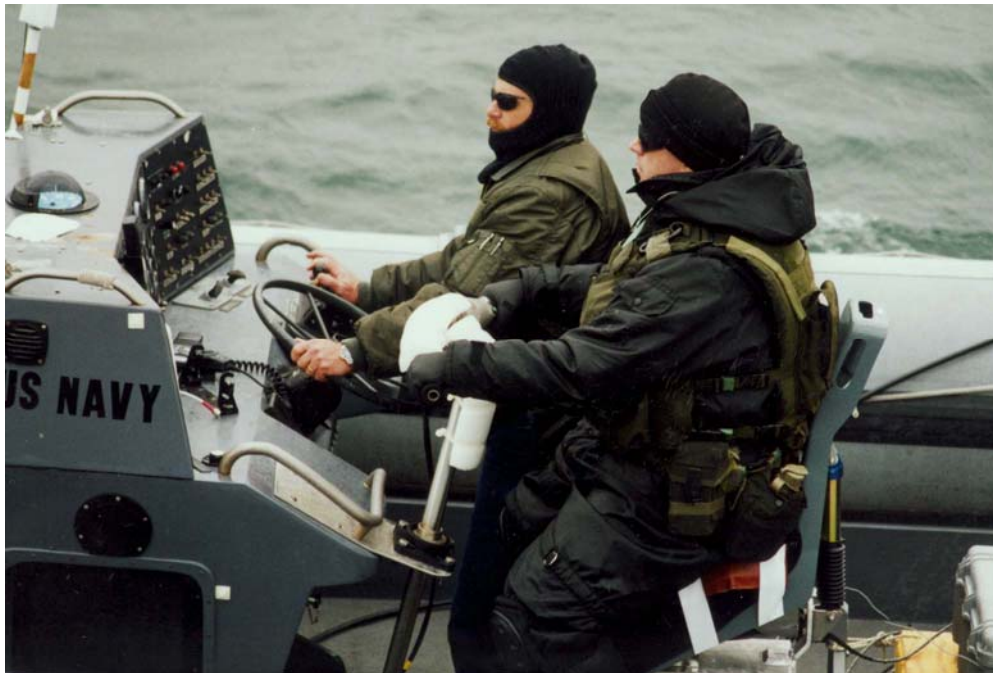
Figure 2: Ullman Cockpit (in foreground) and baseline cockpit (in background). For the tests cockpits were mounted side by side.
